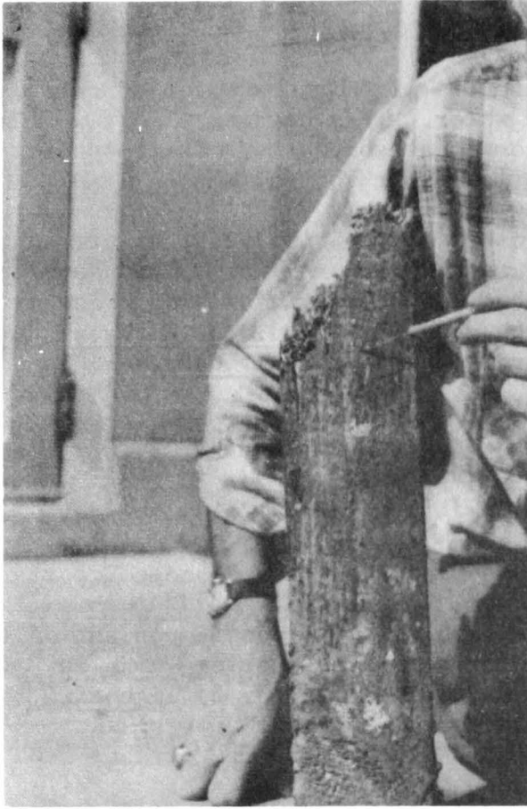
Portion of piling infested with shipworms. Dissecting needle indicates the small entrance to a shipworm burrow.
